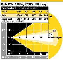
Beam angles-points at which intensity drops to 50% of maximum
